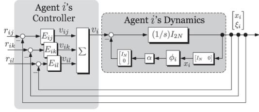
Fig. 2. Block diagram of agent  $i$ 's dynamics for unconstrained optimization. The system enclosed by the dashed line is passive from  $\bar{v}_i$  to  $[\bar{x}_i^T \bar{\xi}_i^T]^T$  (Lemma 4), where  $\bar{v}_i$ ,  $\bar{x}_i$  and  $\bar{\xi}_i$  are defined in (11) and (12).
