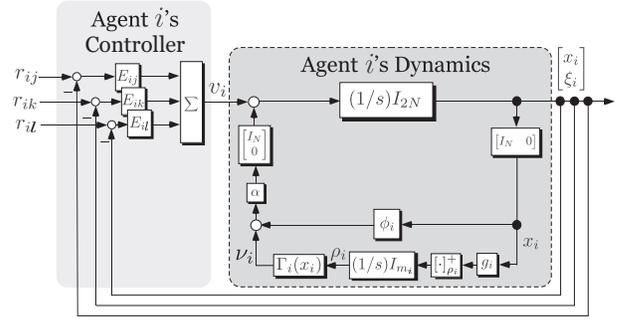
Fig. 3. Block diagram of agent  $i$ 's dynamics for the constrained optimization in the presence of communication delays. The system enclosed by the dashed line is passive from  $\bar{v}_i$  to  $[\bar{x}_i^T \bar{\xi}_i^T]^T$  (Lemma 8), where  $\bar{v}_i$ ,  $\bar{x}_i$  and  $\bar{\xi}_i$  are defined in (11) and (12).
