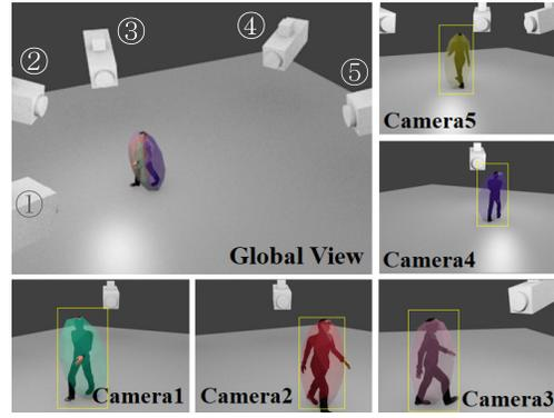
Fig. 4. Intended scenario of 3-D visual human localization. Each camera acquires a rectangle enclosing the human (yellow boxes in the small windows) using a pedestrian detection algorithm. The transparent colored ellipsoids in the small windows are final estimates generated by the algorithm presented in Section IV, and all of them are also shown in the large window.
