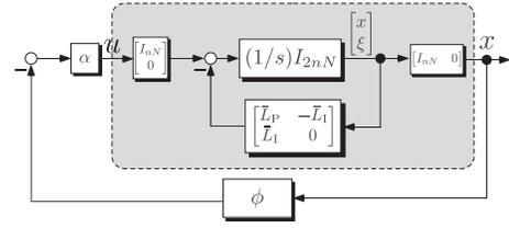
Fig. 1. Block diagram of the PI consensus-based distributed optimization algorithm for unconstrained optimization. The system enclosed by the dashed line is passive from  $\tilde{u} = u - u^*$  to  $\tilde{x} = x - x^*$  with  $x^* := \mathbf{1}_n \otimes z^*$  and  $u^* := -\alpha\phi(x^*)$  (Lemma 3). The bottom block  $\phi$  is incrementally passive (Lemma 1), and hence passive from  $x - x^*$  to  $\phi(x) - \phi(x^*)$ .
