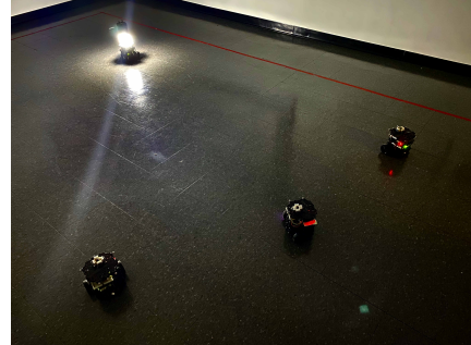
Fig. 1: A snapshot of seeking a moving light source in a dark room with three mobile light sensors.
